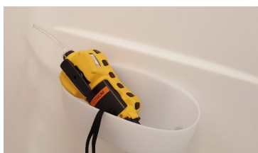
Figure 14. The device in the shampoo/soap holder above the tub during the wet contact time phase.
