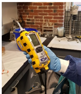
Figure 12. MultiRAE PID device used to measure airborne chlorine.
